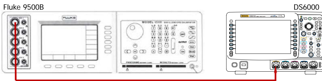
Figure 2-5 Time Base Accuracy Test Connection Diagram
