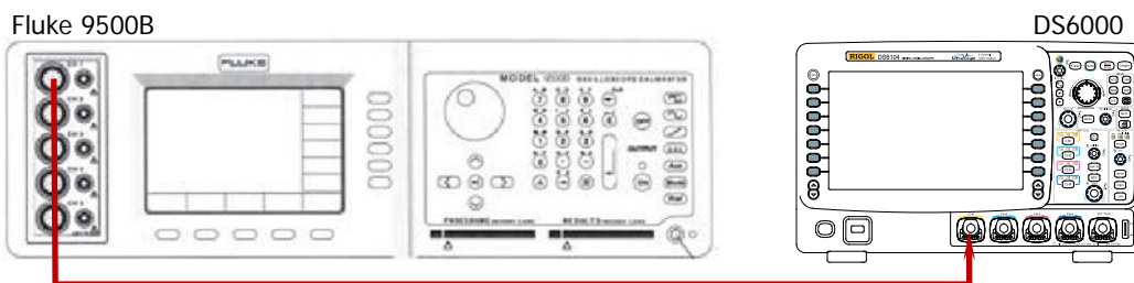
Figure 2-3 Bandwidth Test Connection Diagram
