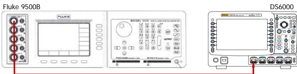
Figure 2-6 Zero Point Offset Test Connection Diagram
