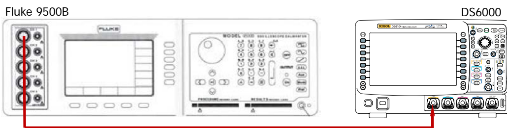
Figure 2-1 Impedance Test Connection Diagram
