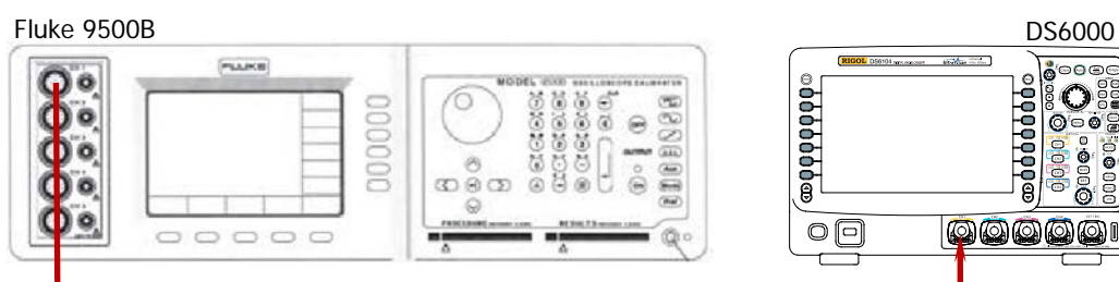
Figure 2-2 DC Gain Accuracy Test Connection Diagram
